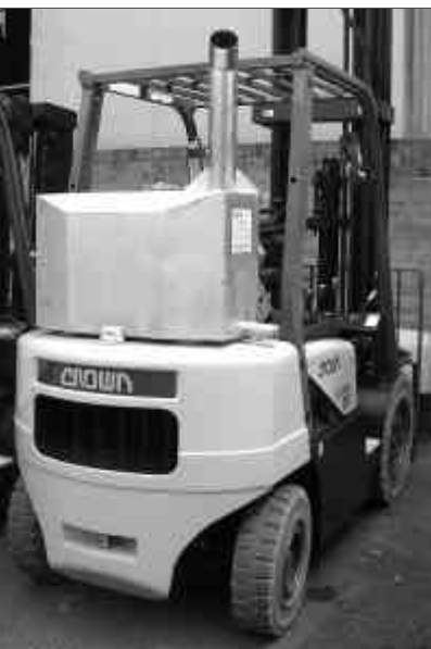
High grade austenitic stainless steel is used to manufacture exhaust scrubber tanks fitted to diesel forklifts used in hazardous areas. The interaction of the exhaust fumes and water produces a corrosive solution requiring the water to be changed daily. Each tank is fitted with a sacrificial anode to prolong the tank's life.
