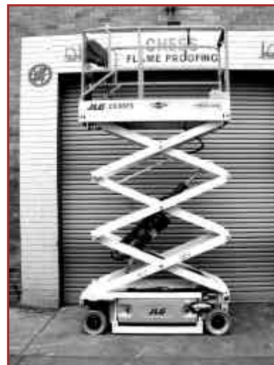
Images of a mobile vertical lift and a scissors lift recently modified for use in Zone 22 (dust) hazardous areas.
